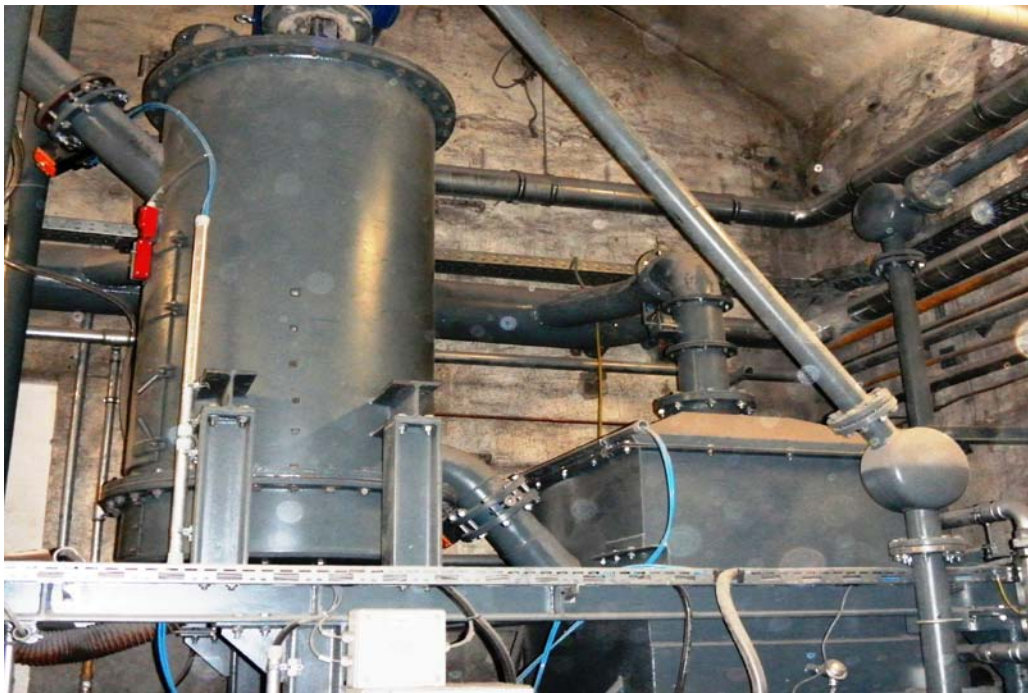
Fig. 5 cleaning unit (6) with oscillating cooling conveyor (7) on right hand side
