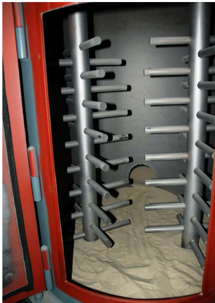
Fig. 6 Interior of cleaning unit (6) with new agitation kits
