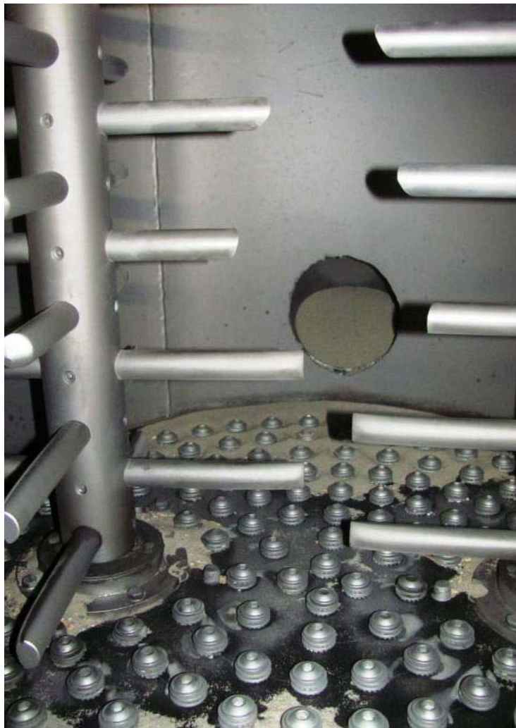
Fig. 7 cleaning unit (6); Nozzle floor with used agitation kits
