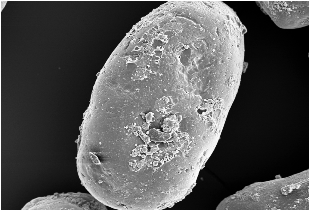
Fig. 8 Reclaimed sand from surge device (5); REM-Microscopy; Magnification 160:1
