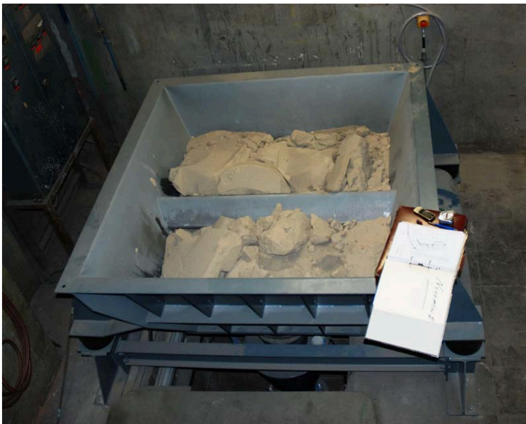
Fig.2 Vibrating sand lump crusher (3) with cast sand moulds
